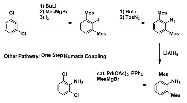
Scheme 3. Improved synthesis of the phosphorus-based biradicaloid precursor.
