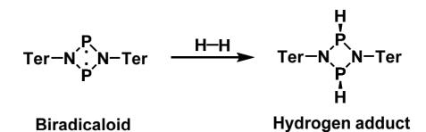
**Scheme 1.** Synthesis of the potential hydrogen transfer reagent.
