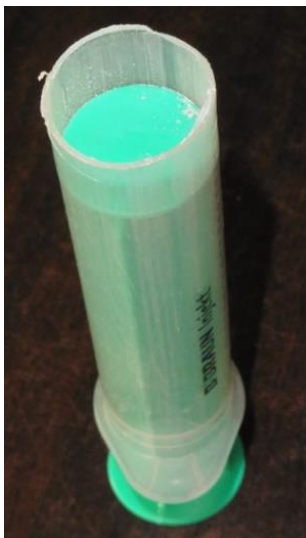
Fig. 3.2-7 As miniature-sampling tube prepared 20 ml syringe.
