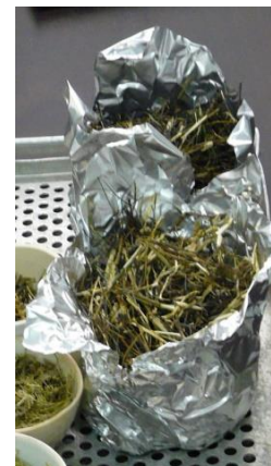
Fig. 3.2-6 Large dry matter in aluminium foil packed for ashing
