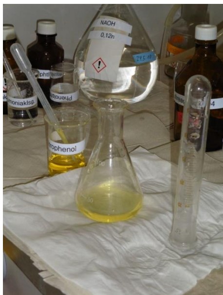
Figure 4.1.5-1 Yellow solution (nitrophenol) after addition of ammonia solution
