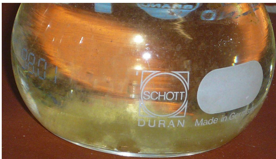
Fig. 4.4.1-1 Precipitation of the ferrihydrite after the digestion of a ferrous samples
